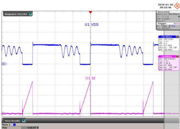
Figure 44 – Drain Voltage and Current Waveforms. 180 VAC, 9.0 V, 3.3 A Load, (419 V MAX ). Upper: V DRAIN , 200 V, 5 μs / div. Lower: I DRAIN , 0.5 A / div.
