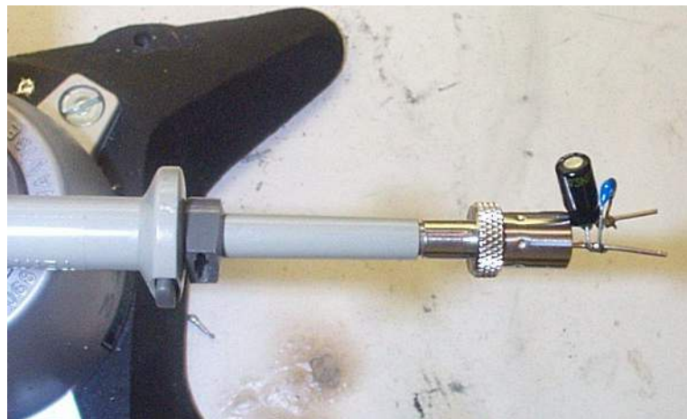
Figure 67 – Oscilloscope Probe with Probe Master ( www.probemaster.com ) 4987A BNC Adapter. (Modified with wires for ripple measurement, and two parallel decoupling capacitors added)
