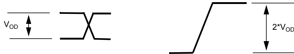
Figure 19 - Differential Output Voltage Parameter
