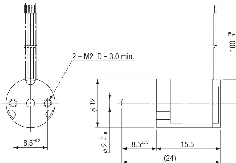
Unless otherwise specified, tolerance : ± 0.4 (Unit : mm)
