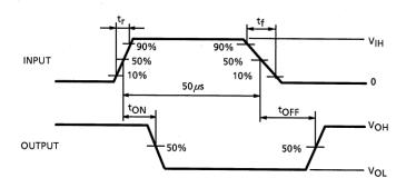
Note 1: Pulse width 50 μs, Duty cycle 10%
