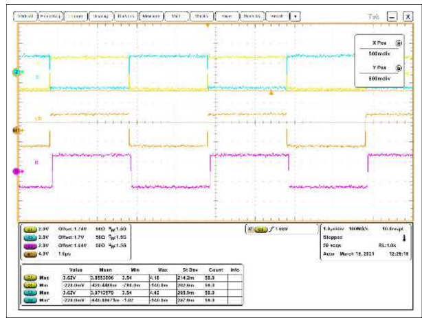
Figure 8-20. ISOW1412 Driver Propagation Delay - RS485 Mode
