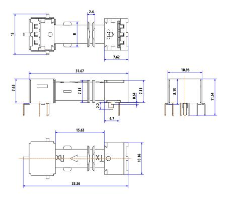
NOTE: Dimensions are in millimeters (mm).
