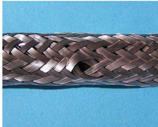
NOTACCEPTABLE Window in Shield
