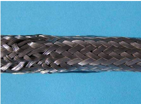
NOTACCEPTABLE Uneven Coverage
