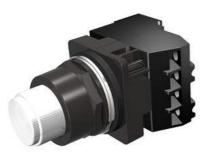
30mm BlackMax, Epoxy Coated Corrosion Resistant Complete Metal Unit PTT / Illuminated Pushbutton Transformer type, 600V AC LED Lamp Extended Button Plastic Lens, White 2 Position Momentary with 1 N.O. - 1 N.C. Heavy Duty Contacts, A600/P600 UL Listed, CSA Certified NEMA 1,3,3R,4,4X,12,13 & Automotive Standards
