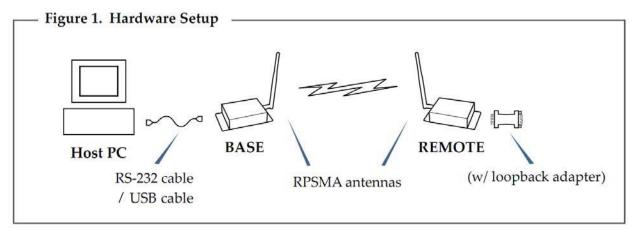
Note: To run a successful range test, the remote end must be an RS-232 device.
