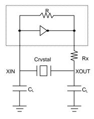
$\begin{array}{l} C_L = 2^*(C_P - C_S), \\ \text{Where } C_P = \text{Load capacitance of crystal from crystal vendor datasheet.} \\ C_S = \text{Stray capacitance due to } C_{\text{IN}}, \text{PCB}, \text{Trace, etc.} \end{array}$
