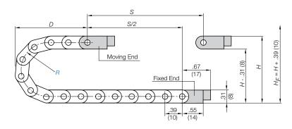
Supplement part number with required radius. Example: E03-05-028-0 Pitch: .39 in. (10 mm) per link links/ft (m) = 30.47 (100)
