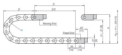
Pitch per link: = .39" (10 mm) Links per ft (m): = 30.47 (100) For center mount applications: Chain length =  $_{\rm s}^{9/2}$  + K
