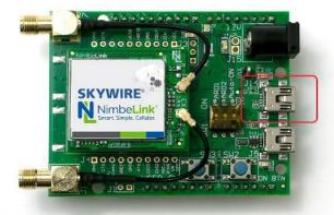
The USB to serial UART IC is an FTDI FT234XD. The FTDI drivers for the FT234XD are available on FTDI's website.
