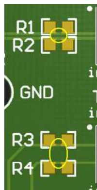
Figure 5. R1, R2, R3 and R4 shorting traces must be cut before use
