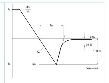
Fig. 6. Reverse recovery definitions; ramp recovery
