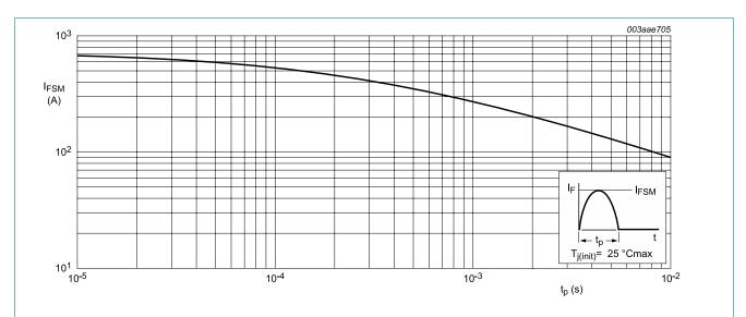
Fig. 3. Non-repetitive peak forward current as a function of pulse width; sinusoidal waveform; maximum values
