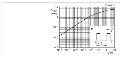
Fig. 4. Transient thermal impedance from junction to heatsink as a function of pulse width
