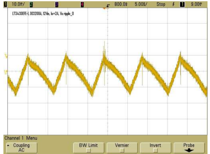
Figure 4. Typical VOUT ripple 12VIN 2A load
