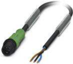
Sensor/Actuator cable, 3-position, PUR halogen-free, Black-gray RAL 7021, Plug straight M12, A-coded, on Free cable end, Cable length: 3 m, with plastic knurl
