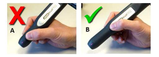
While plasma is being generated, do not put your hand into the working area. This may disturb the plasma discharge and cause skin irritations and might be slightly painful.
