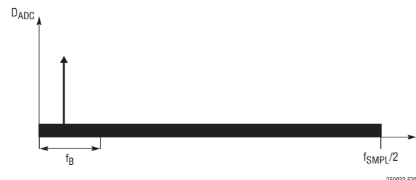
Figure 20. Frequency Spectrum of SAR ADC Core Output
