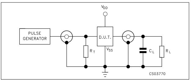
$C_L$  = 50pF or equivalent (includes jig and probe capacitance)  $R_L$  = 200KΩ  $R_T$  =  $Z_{OUT}$  of pulse generator (typically 50Ω)
