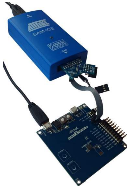
Figure 5-7. SAM-ICE using an Atmel-ICE Adapter
