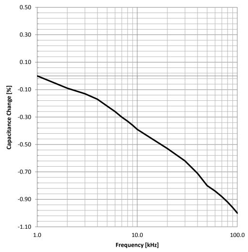
Test Equipment: E4991A or equivalent
