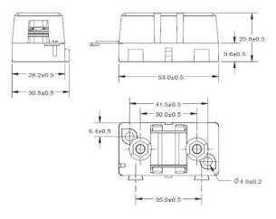
Bolt size M5, recommended torque 3.5 - 4 N-m
