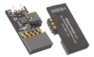
TIMI requires the jumper to be positioned like the image above, closest to the 5-way female header. This makes the programmer compatible with programming the 4D Labs Pixxi28 processor.
