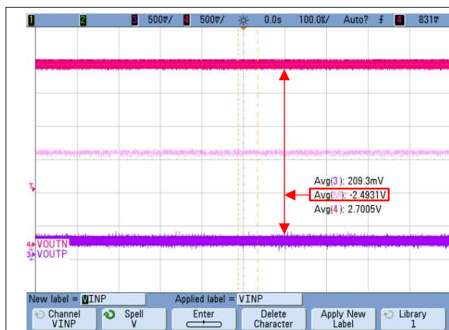
Figure 50. Typical Negative Clipping Output of the AMC1302-Q1
