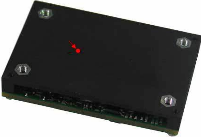
Figure 16 Test point on baseplate
