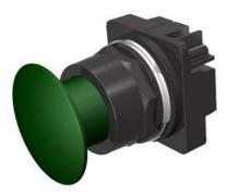
30mm BlackMax, Epoxy Coated Corrosion Resistant Metal Operator, Round Push-Pull Operator Non-Illuminated Mushroom Head Cap Small 1.73" (44 mm) Metal, Anodized Green 3 Position Pull-Momentary/Push-Maintained UL Listed, CSA Certified NEMA 1,3,3R,4,4X,12,13 & Automotive Standards
