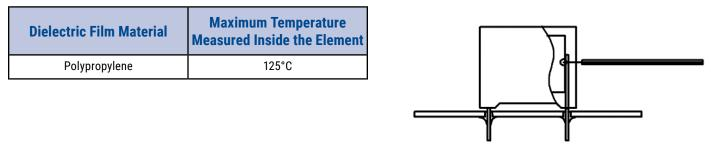
Temperature monitored inside the capacitor.
