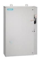
Non-reversing motor starter Size 1 Three phase full voltage Solid-state overload relay OLRelay amp range 3-12A 24VAC 50-60HZ coil Combination type 30Amp non-fusible disconnect Encl NEMA type 4X 316 S-steel Water/dust tight non-corrosive Extra-wide enclosure
