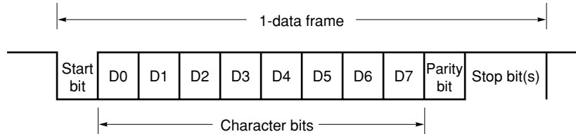
Figure 16-7. Format of Asynchronous Serial Interface Transmit/Receive Data
