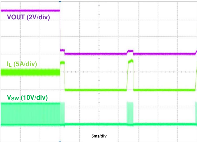
Figure 21. Output Short Protection, IOU = 5A
