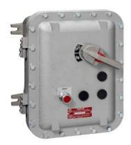
Non-reversing motor starter, Size 2 1/2, Three phase full voltage, Solid-state overload relay, OLRelay amp range 25-100A, 110V 50HZ / 120V 60HZ coil, Combination type, 100A non-fusible disconnect, Encl. NEMA type 4X Fiberglass Water/dust tight noncorrosive, Standard width enclosure
