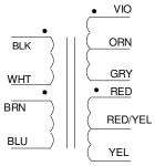
Input: Series – BLK to BLU, Jumper WHT to BRN Parallel – BLK to BLU, Jumper BLK to BRN and WHT to BLU Output: Series – VIO to YEL, Jumper GRY to RED Parallel – VIO to YEL, Jumper VIO to RED and GRY to YEL
