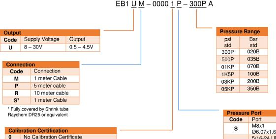
The psi range models are only supplied with imperial thread design. The bar range models are only supplied with metric thread design
