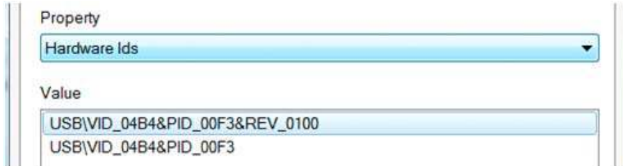
Figure A-2. Default FX3 Bootloader VID/PID
