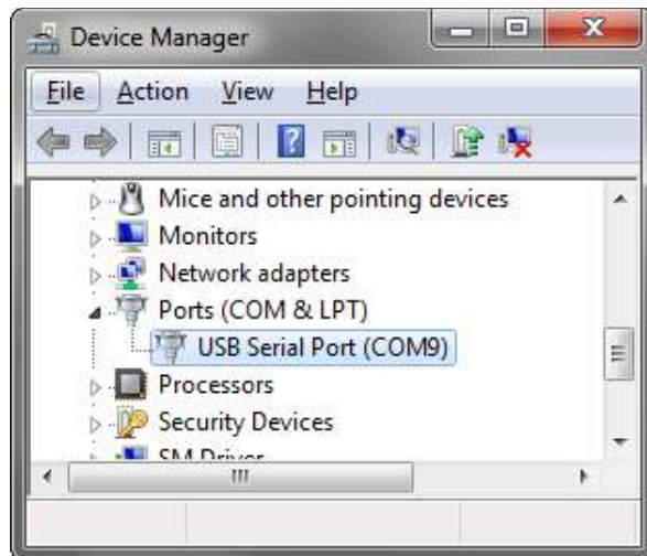
Figure 3-16. USB Serial IC Enumerating as COM Port
