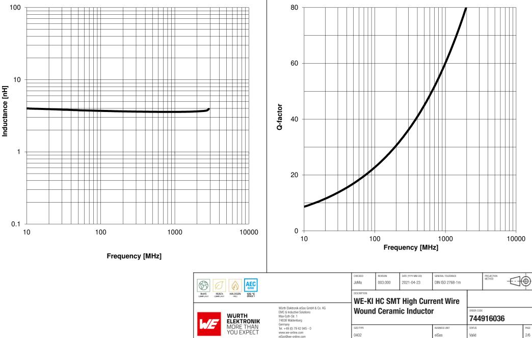
**Typical Inductance vs. Frequency Characteristics:**
