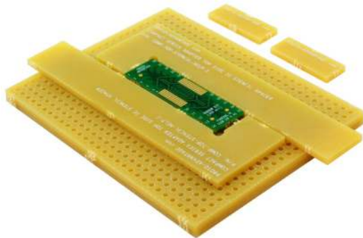
Image 3: Spacer stack with compact adapter in place, ready for stencil to be taped down on top.
