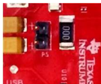
Figure 2-13. Current Measurement Point
