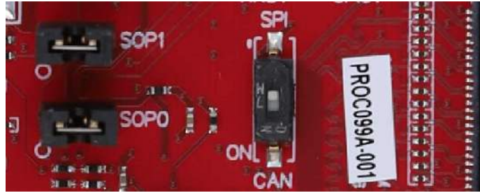
Figure 2-14. S1 Switch to Select Between SPI or CAN Interface
