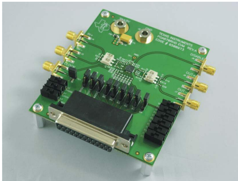
Figure 1. Switch and Jumper Block Positions for Enabled Device, Gain = 20 dB, Unlatched Gain Mode
