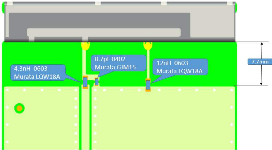
Ground clearance dimensions (mm) and matching component values
