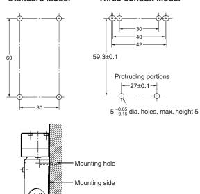
The D4BS can be mounted more securely by adding two protruding portions, each of which is 5 mm maximum in height and 5  $^{-0.05}/_{-0.15}$  mm in diameter as shown below.
