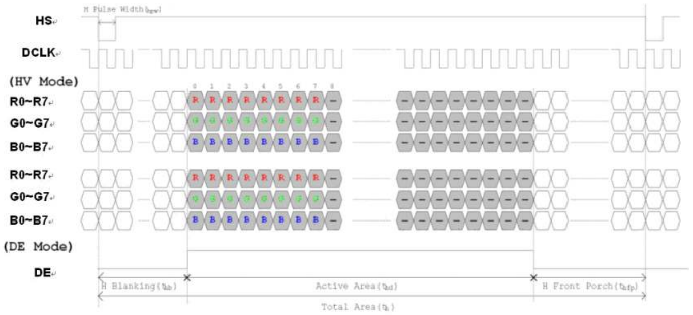
Figure 5: Horizontal Input Timing Diagram
