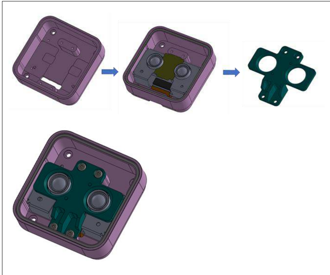
Figure 7-15. Stereo Depth Module Mid-Mounting – D401
