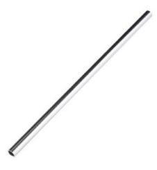
**Description:** These 10" long aluminum tubes have an outer diameter of 3/8", an inner diameter of 0.30", and a wall thickness of 0.035". When used with the mating tube clamps, these can be used for versatile structural support. Additionally, wires and cables can easily be run through the center.
