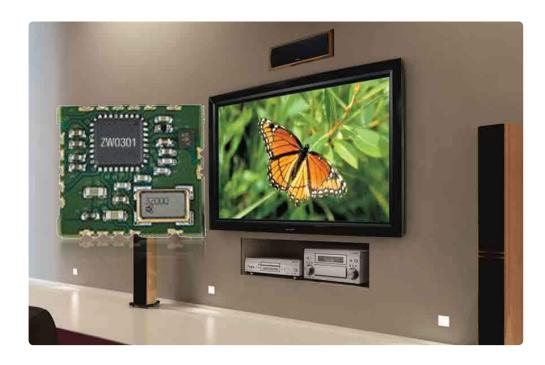
The ZM3102 represents the third-generation of Z-Wave® wireless technology, and is ideal for easily adding Z-Wave® control and status capabilities to home control, home security monitoring, and home energy management products. The ZM3102 module includes a Z-Wave® chip and external components required to implement a complete, drop-in solution.
