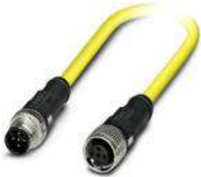
Sensor/Actuator cable, 5-position, TPE, yellow RAL 1021, Plug straight M12 SPEEDCON, A-coded, on Socket straight M12 SPEEDCON, A-coded, Cable length: 1.5 m
