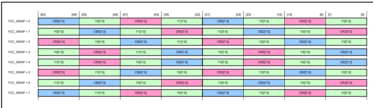
Figure 35.6 YCbCr422 Data Arrangement with Swapping Enabled
