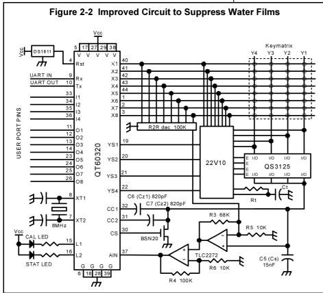
Vgs. The mosfet should have an input capacitance (Ciss) of under 50pF for low charge injection.
