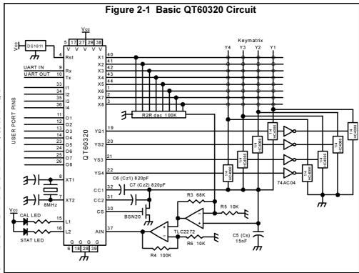
If there is a large amount of coupling between X and Y lines, and where burst length 'n' is set to a high number, charge accumulation on Cs may reach a point where the ladder DAC can no longer offset the signal back into the ADC's usable range. In this case the circuit will employ one or two of the Cz capacitors to 'knock back' or cancel the charge accumulated
