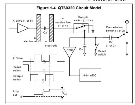
subtract charge from Cs to create a negative-going offset, bringing the signal back to a usable level. This action occurs during the course of the burst and is not illustrated in the timing diagram of Figure 1-4. This mechanism has the benefit of allowing high levels of Cx while remaining highly sensitive to small changes in charge coupling due to touch; the circuit permits the designer to create very large, highly interdigitated touch keys that are very sensitive.
