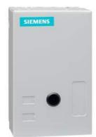
Non-reversing NEMA contactor, Size 0, Single phase full voltage, Contactor amp rating 18A, 3 wire (NO aux included), 208VAC 60Hz coil, Non-combination type, Enclosure NEMA type 1, Indoor general purpose use, Standard width enclosure
