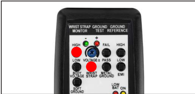
Figure 12. Pressing the WRIST STRAP and HIGH BODY VOLTAGE test switches simultaneously
