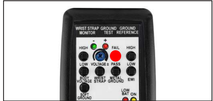
Figure 22. Pressing the METAL GROUND FAIL test switch
