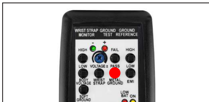
Figure 16. Pressing the METAL GROUND PASS test switch
