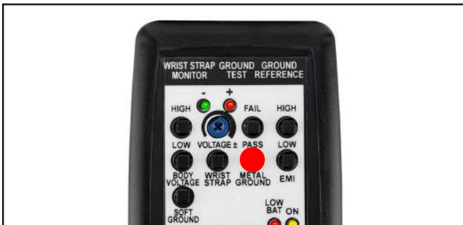
Figure 21. Pressing the METAL GROUND PASS test switch
