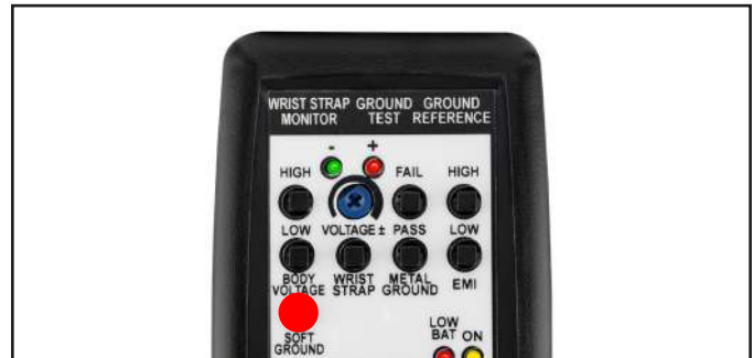
Figure 14. Pressing the SOFT GROUND test switch
