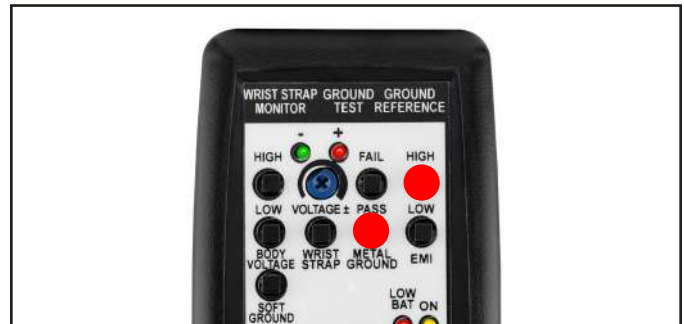
Figure 24. Pressing the METAL GROUND PASS and EMI HIGH test switches simultaneously
