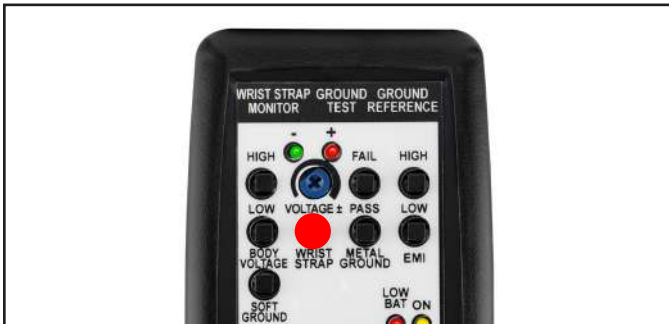
Figure 4. Pressing the WRIST STRAP test switch
