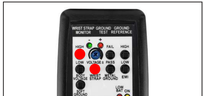
Figure 28. Pressing the WRIST STRAP and HIGH BODY VOLTAGE test switches simultaneously
