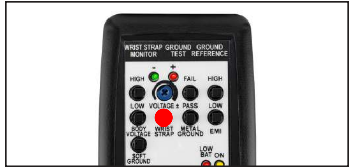
Figure 26. Pressing the WRIST STRAP test switch
