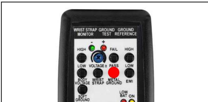
Figure 30. Pressing the METAL GROUND PASS test switch
