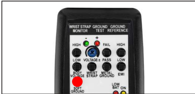
Figure 8. Pressing the SOFT GROUND test switch
