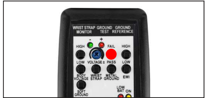
Figure 17. Pressing the METAL GROUND FAIL test switch
