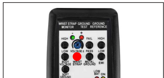
Figure 10. Pressing the WRIST STRAP test switch
