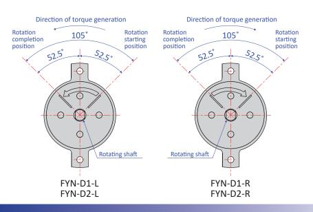
• The damper's working angle is 105° with respect to the attachment flange, as shown to the left. Please determine where to attach it according to your needs. Also, rotating the damper beyond this angle will cause damage to the damper. Please ensure that an external stopper is in place.
